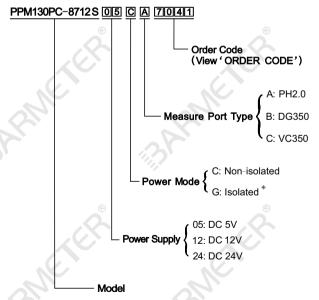
When choose isolated power mode, signal's unbalanced input cannot be used.
